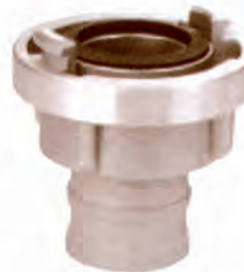
HC-227 Storz Couplings Aluminium Alloy/Brass-Forged Storz25-DIN14306 Storz52-DIN14307 Storz65-NEN3374 Storz75-DIN14308
